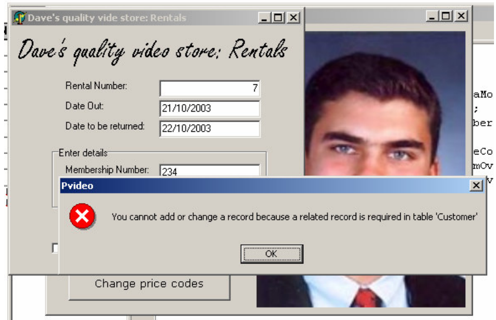
Figure 3 → Referential integrity generates error as Customer #234 does not exist.
